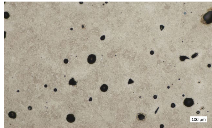
As quenched and tempered (oil quenched +300 °C, 1 h)
